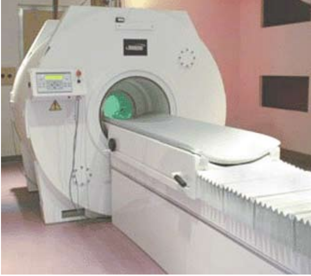
▲ The 3.0 Tesla head-only MRI system used in our research, located at the Lawson Health Research Institute, St. Joseph's Health Centre, London, ON.
